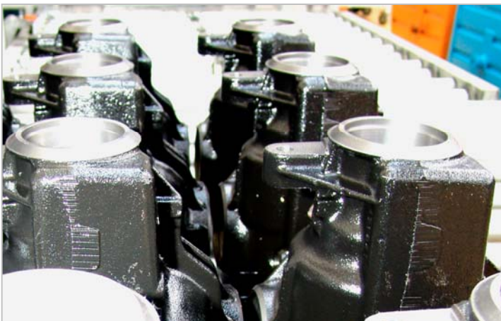
Demanding task: The gearbox is fully machined on 2 Mazak machining centres
