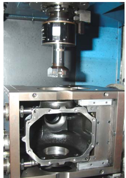
Today, the internal machining of the two grooves is accomplished in a single operation – the machining time dropped from 120 to only 40 seconds
